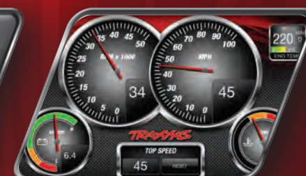
Telemetry Sensors Installed View speed, RPM, temperature, and voltage data on the Traxxas Link dashboard
